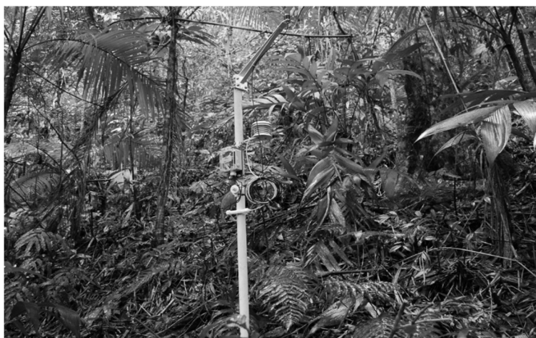
Figure 3: Weather station composed of HOBO H21 data logger, installed in the understory, collecting data of temperature ( ^\circ\text{C} ) and relative humidity (%).
