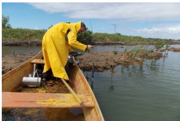
Figure 2: Data collection with the multiparametric probe in the Ipiranga River, at the sampling area RIO 4 (423093.00 m E7890925.00 m S).
