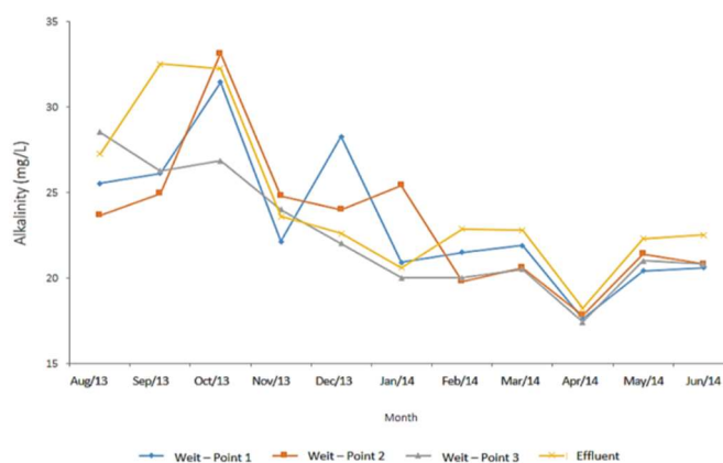
Figure 8: Graph of the values of alkalinity verified in the supply and effluent weir of the Carlos Eduardo Matiazze Fish Farming Center, Presidente Médici/RO, Brazil.
