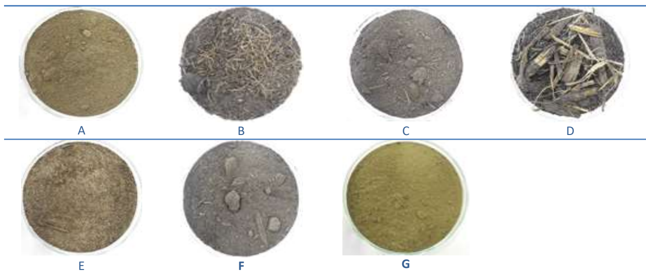
Figure 2: Visual characterization of the material retained in 4,000 μm sieve revealing coarse material in seven samples of ash collected in sugarcane industries of Mato Grosso do Sul.
