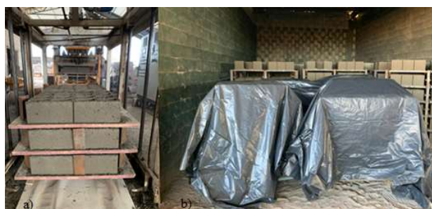
Figure 5: a) Manufacture of blocks; b) Cure using canvas.
