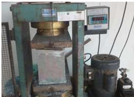
Figure 6: Compressive strength test.
