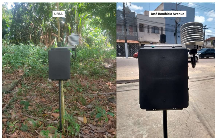
Figure 6: Sensory Platform fixed, in a height of 1.5 meters from the floor.
